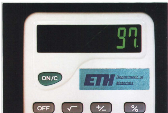
Figure 4. (a) Photograph of a PL display device according to Figure 3a. (b) Photograph of a bicolor device according to Figure 3b. (Figure 4a reproduced with permission from ref. 31.) Copyright 1998 American Association for the Advancement of Science.
