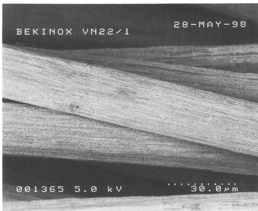
Figure 3. Photomicrograph of a circa. 20 micron diameter stainless steel fiber at 1000X magnification.
